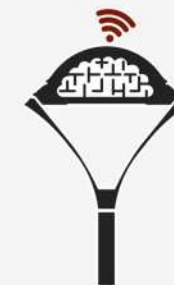
Meshed network radio system where each smart luminaire acts as a receptor/transmitter to and from the control centre.
